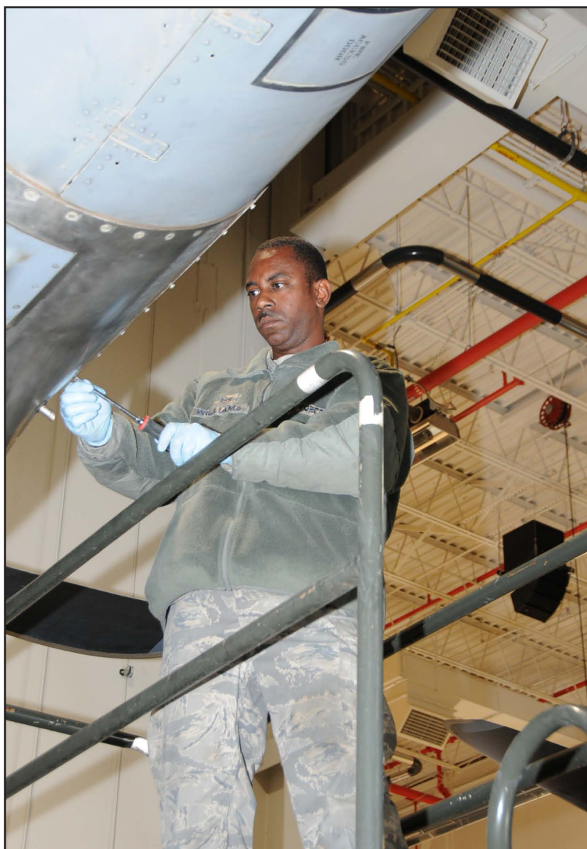
Tech. Sgt. Meceikee Williams, Aerospace Propulsion, aircraft engine mechanic, works to remove a panel to expose an engine of an aircraft as part of post deployment cleaning. The Aerospace Propulsion shop was assessed by a team of 25 inspectors as a part of the Logistics Compliance Assessment Program inspection of the Maintenance Group (Photo by Senior Airman Claire Behney).
